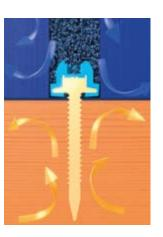
A combination of hot box tests and thermal activity recording at EJOT's testing centre Applitec, has repeatedly shown that the composition of the Opticore head provides significantly better thermal retention values over allmetal fastenings.
