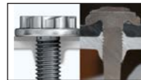
The polygonal point and the conical thread-forming zone ensure easy flow drilling through heating up of the material.
