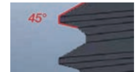
The asymmetric 45° flank angle causes smaller material displacement compared to common 60° threads and results in higher strength of the joint.
