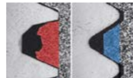
The asymmetrical flank angle of 33° guarantees much higher strength values of the formed female thread root than a common 60° thread.
